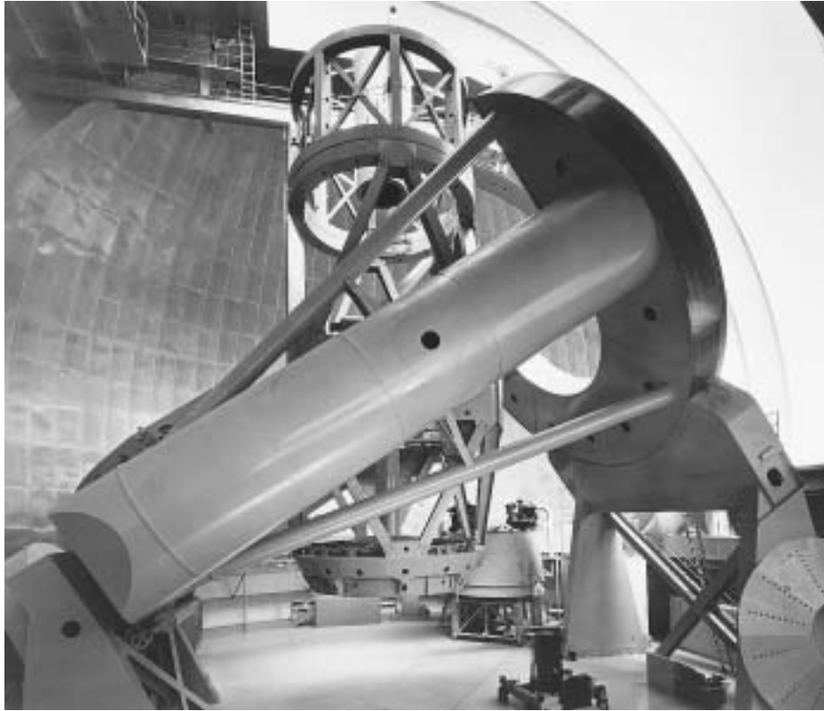
FIGURE 2.43 Palomar Observatory, located on Palomar Mountain in southern California, houses the 200-inch Hale reflecting telescope.
