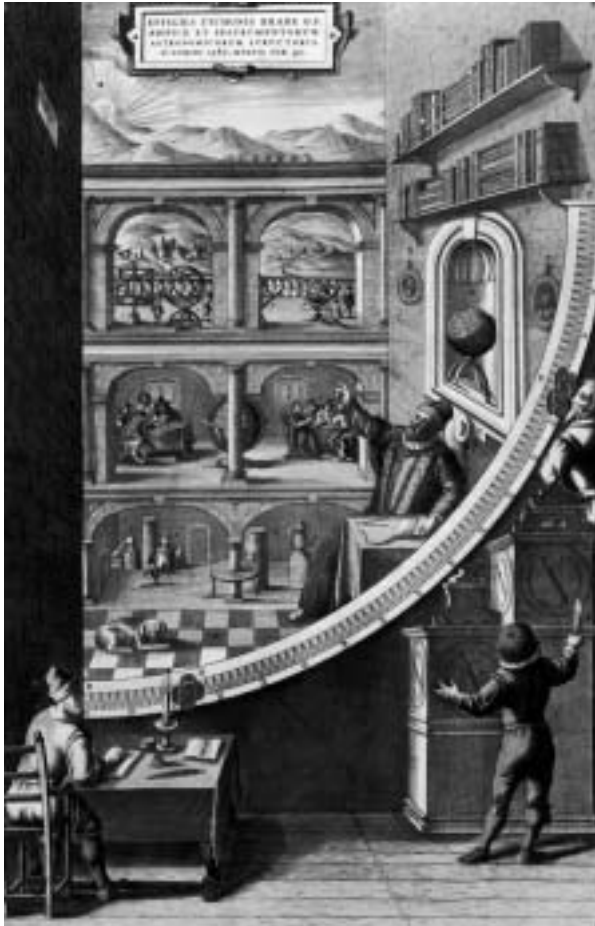
FIGURE 2.27 The hall containing Tycho Brahe's great quadrant. The rest of the laboratory is shown, with Brahe making an observation (aided by assistants).
